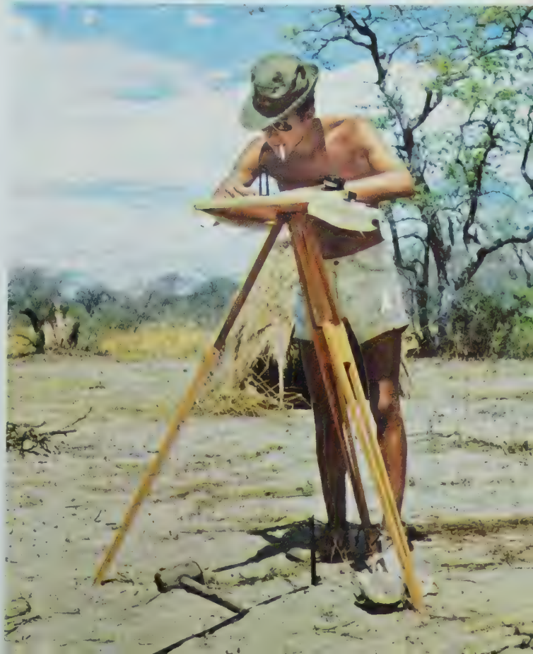
PLOTTING A VILLAGE SITE, photographer Stanley Washburn uses a plane table on which all dwellings and their human appurtenances will be marked with the precision of a surveyor.
