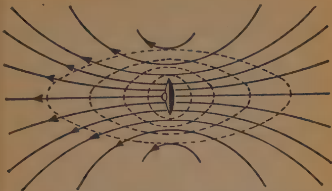
Figure 9. Principle of Plantier's force field. The curved arrows symbolize the lines of force. The dotted ellipses represent the ellipsoidal surfaces of equal field intensity.
